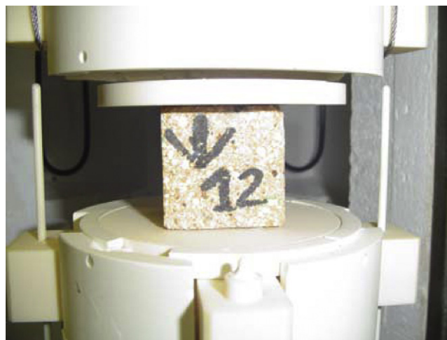
Fig. 2. View of a prefired BSAA sample in the uniaxial compression set-up during the preparation phase.
