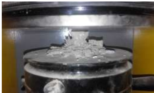
Figure 9b. Brittle failure of fired concrete cubic specimen at room temperature
